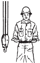
Extend Boom (Telescoping Booms). Both fists in front of body with thumbs pointing outward.
