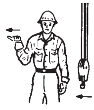
Trolley Travel. Palm up, fingers closed, thumb pointing in direction of motion, jerk hand horizontally.
